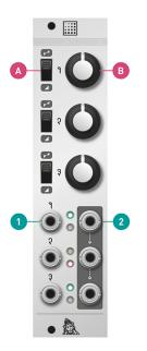
Each of the 3 channels of Shades can act as an attenuator or attenuverter.
