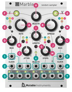
The **t generator** produces random gates by generating a jittery master clock (which is output on  $t_2$ ) and deriving from it two streams of random gates which are output on  $t_1$  and  $t_3$ .
