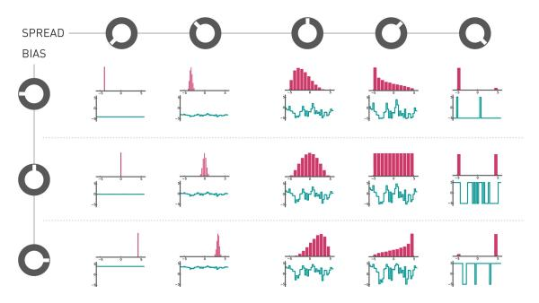
**M. Horizontal and vertical "steppiness"** of the generated voltages. At 12 o'clock, generates the typical S&H steps. Turn CCW to generate smoother edges, then random linear segments, then smooth random curves. Turn CW to quantize the generated voltages to a scale, then to progressively strip the scale of its notes until only the root note remains.
