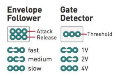
The last setting, corresponding to the longest time or higher voltge, is obtained by removing the jumper.
